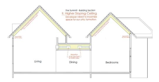
Fig. 2(b): Building section drawing of the Unit
